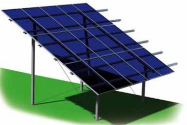
Only energy production system, with double support pole and wind-bracing. THE BASE CONFIGURATION INCLUDES: **2 TO 3 MODULES IN VERTICAL ARRANGEMENT UP TO 6 MODULES IN HORIZONTAL ARRANGEMENT** HMIN max: 1.500 mm HMAX min: 5.000 mm
